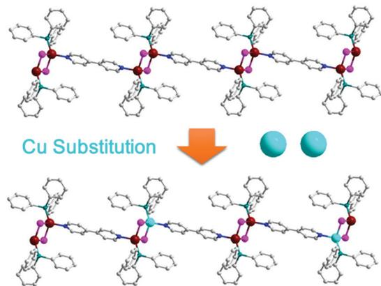
Fig. 1 Illustration of the copper substitution in 1D-Ag<sub>2</sub>I<sub>2</sub>(tpp)<sub>2</sub>(4,4'-bpy). (red ball) Ag; (pink ball) I; (light blue ball) Cu; (gray ball) C; (dark blue ball) N; (green ball) P.
