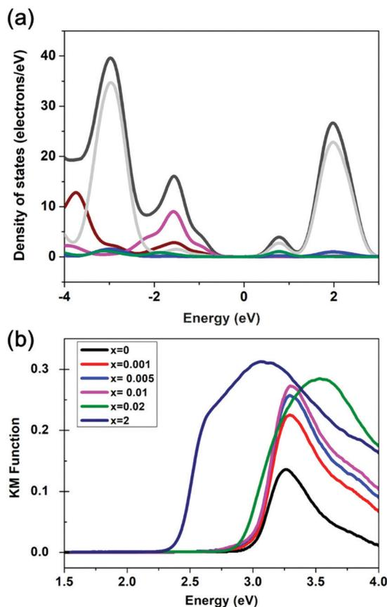
Fig. 2 (a) Calculated density of states (DOS) of **1** by the DFT method: total DOS (black); Ag 4d orbitals (dark red); I 5p orbitals (pink); C 2p orbitals (grey); N 2p orbitals (blue); P 3p orbitals (green). (b) Optical absorption spectra for compounds 1D-Ag<sub>2-x</sub>Cu<sub>x</sub>I<sub>2</sub>(tpb)<sub>2</sub>(4,4'-bpy) ( $x < 2$ ).
