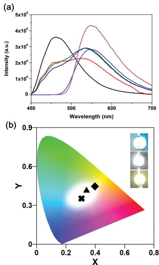
Fig. 3 (a) Photoluminescence spectra of **1** (black), **2** (red), **3** (green), **4** (navy), **5** (blue), and **6** (pink);  $\lambda_{\text{ex}} = 360$  nm. (b) CIE coordinates of **2** (cross), **3** (triangle) and **4** (square). Inset: Photos of the LED bulbs coated by **2–4** under working conditions.
